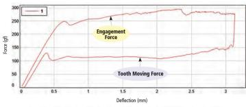
Description: Nickel Titanium .016 – Test Temp: 36 °C – Super Elastic (SE/G4) fully activated by 25°C
